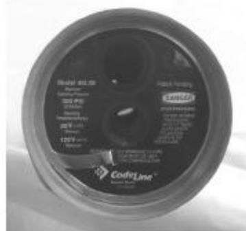
*Retaining ring seated in the groove*
