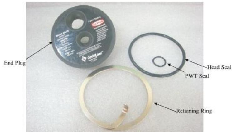
*Head component identification (40L30) Head disassembled*
