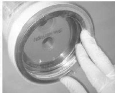
*Inserting Retaining Ring into the groove*
