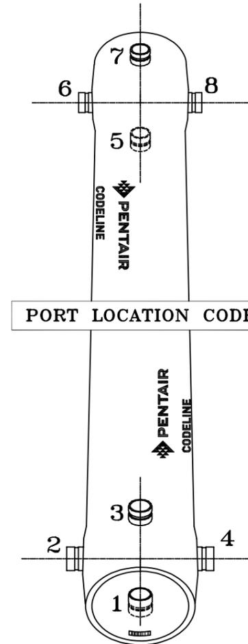
CODELINE BODY LABELS ARE PLACED AT 90° ON SERIAL NUMBER END AND AT 270° ON THE OPPOSITE SIDE END
